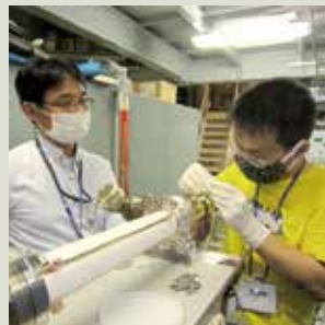
Assembling work of fast beam kicker
