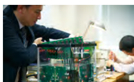
The Cooling Test for Submerging an In-water Computer and Fault-diagnosis Test Boards in Water.
