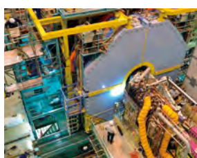
Upgrade of the SuperKEKB accelerator and Belle II detector. ©KEK
