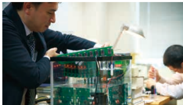
The Cooling Test for Submerging an In-water Computer and Fault-diagnosis Test Boards in Water.
